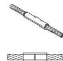
DETALLE SOLDADURA ALUMINOTÉRMICA TIPO I
